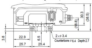
Bottom surface of amplifier mounting bracket
