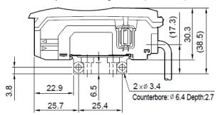
Bottom surface of amplifier mounting bracket
