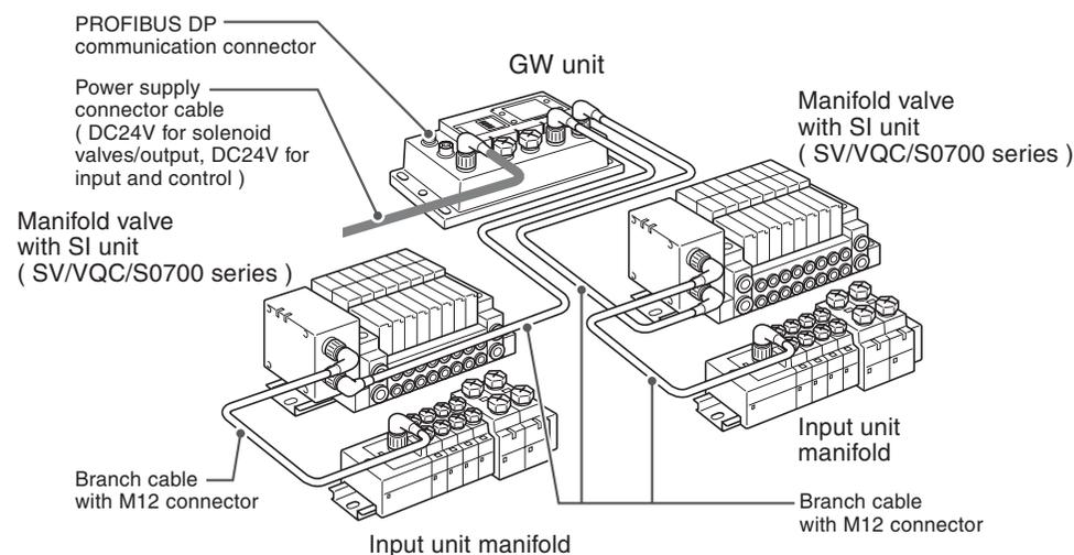
The reduced wiring system is connected to various kinds of fieldbus realizes the reduced wiring and decentralized installation of I/O devices . The signals to/from fieldbus are exchanged by GW unit, and the signals to/from decentralized I/O devices are collected and delivered by GW unit.
